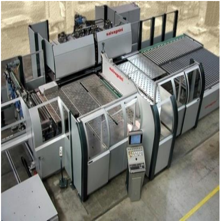
Production line for Wall & Door panel
