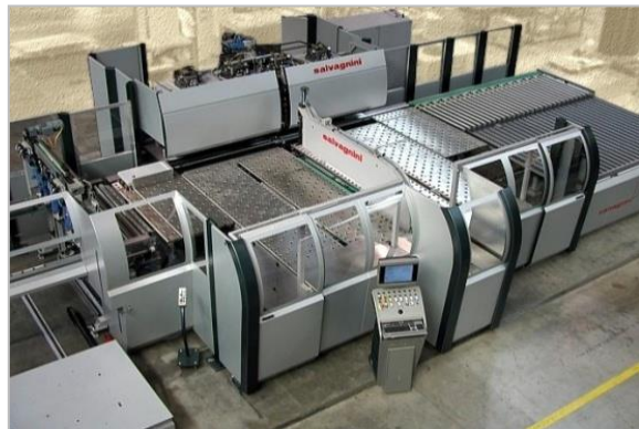
Door panel production line (SALVAGNINI : Italy)
